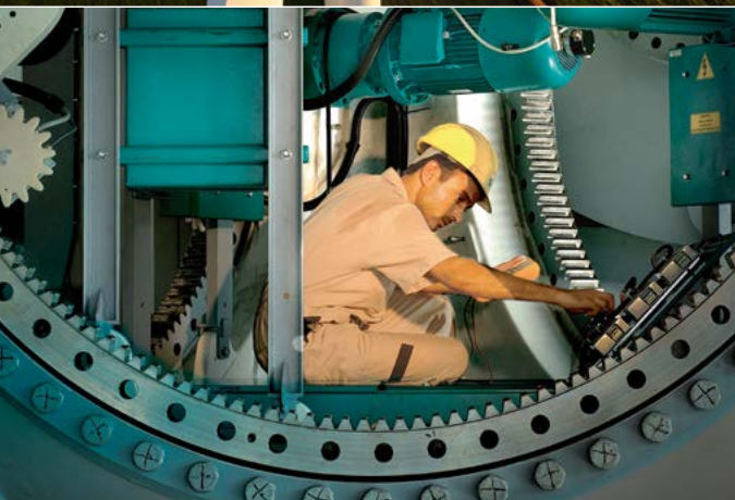
◀ 2 MW-class blade bearing, electric pitch / internal gears
